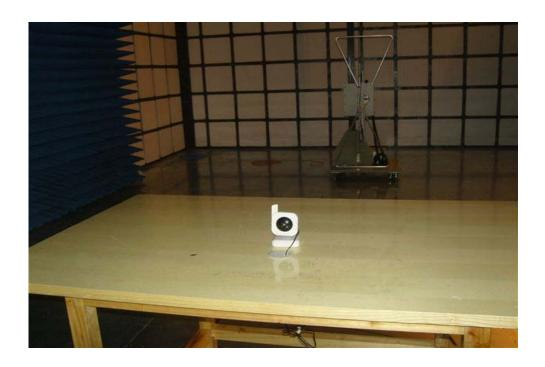
**Radiation Emission Test View For 1GHz-25GHz**
