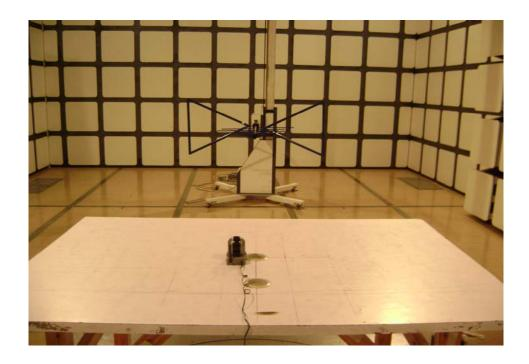
**Radiation Emission Test View For 1GHz-25GHz**
