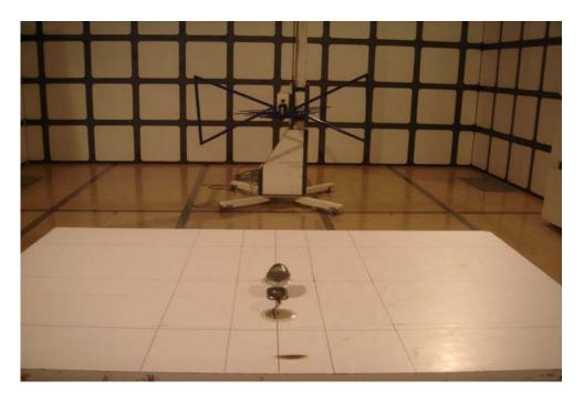
Radiation Emission Test View For 1GHz-25GHz
