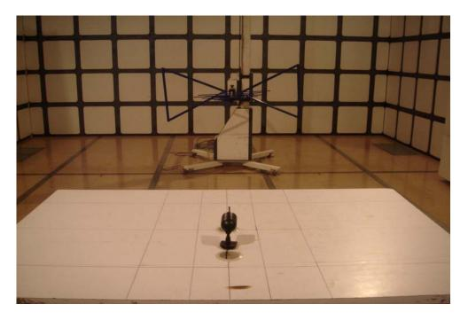
**Radiation Emission Test View For 1GHz-10GHz**
