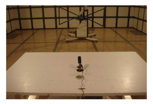
**Radiation Emission Test View For 1GHz-10GHz**
