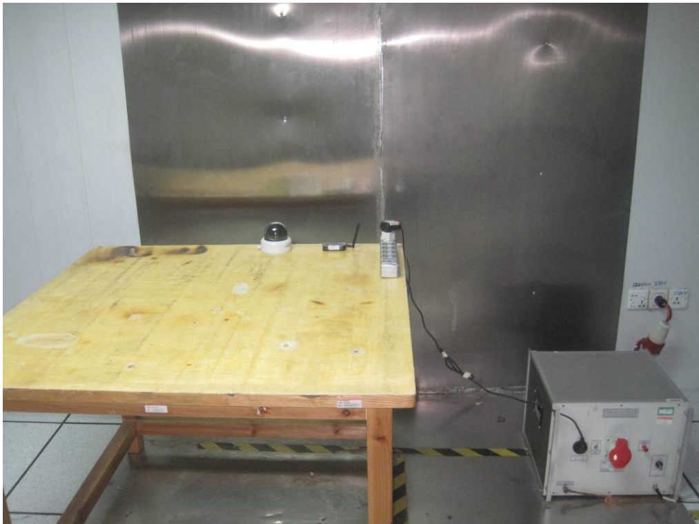
16.2 Photograph – Conducted Emission Test Setup
