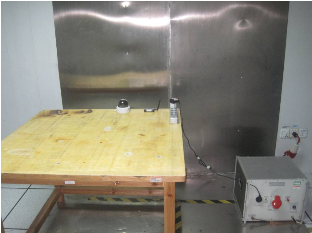
16.2 Photograph – Conducted Emission Test Setup
