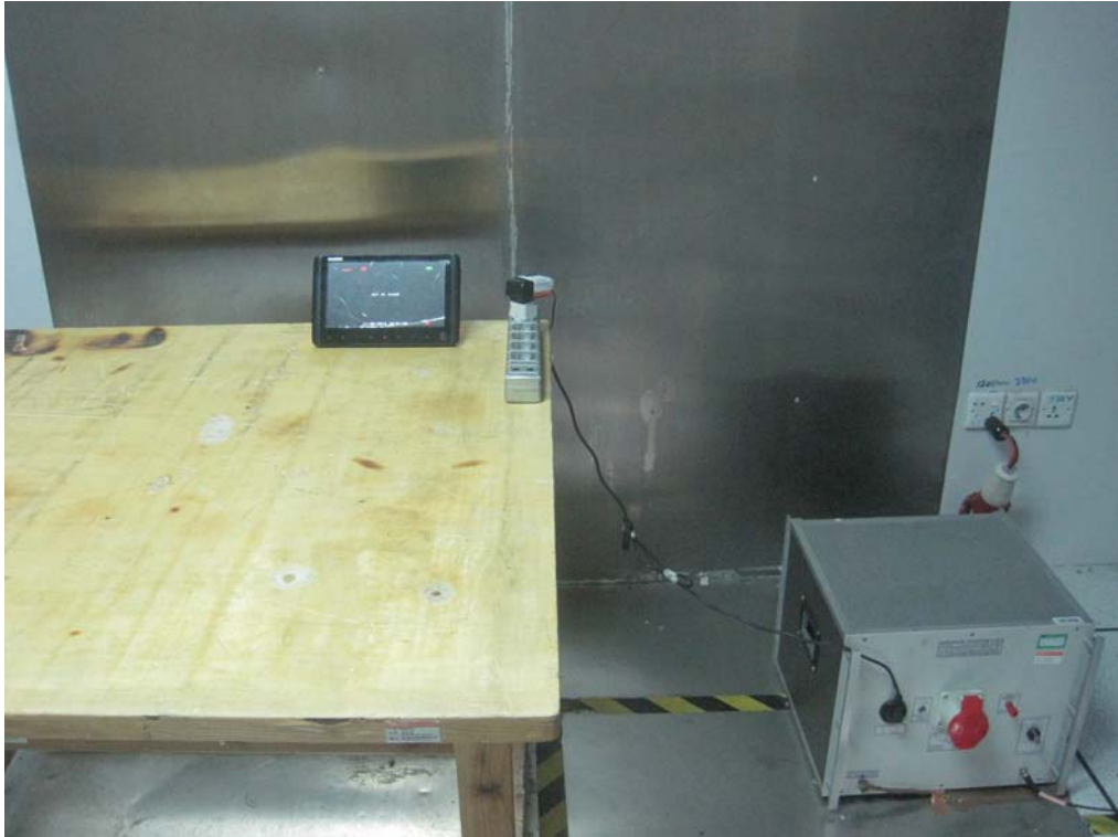
Photograph – Conducted Emission Test Setup
