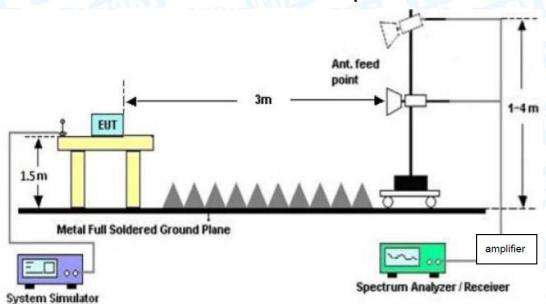
**Above 1GHz Test Setup**
