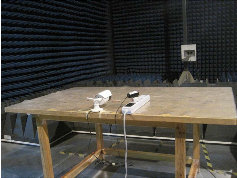
17.2 Photograph – Conducted Emission Test Setup
