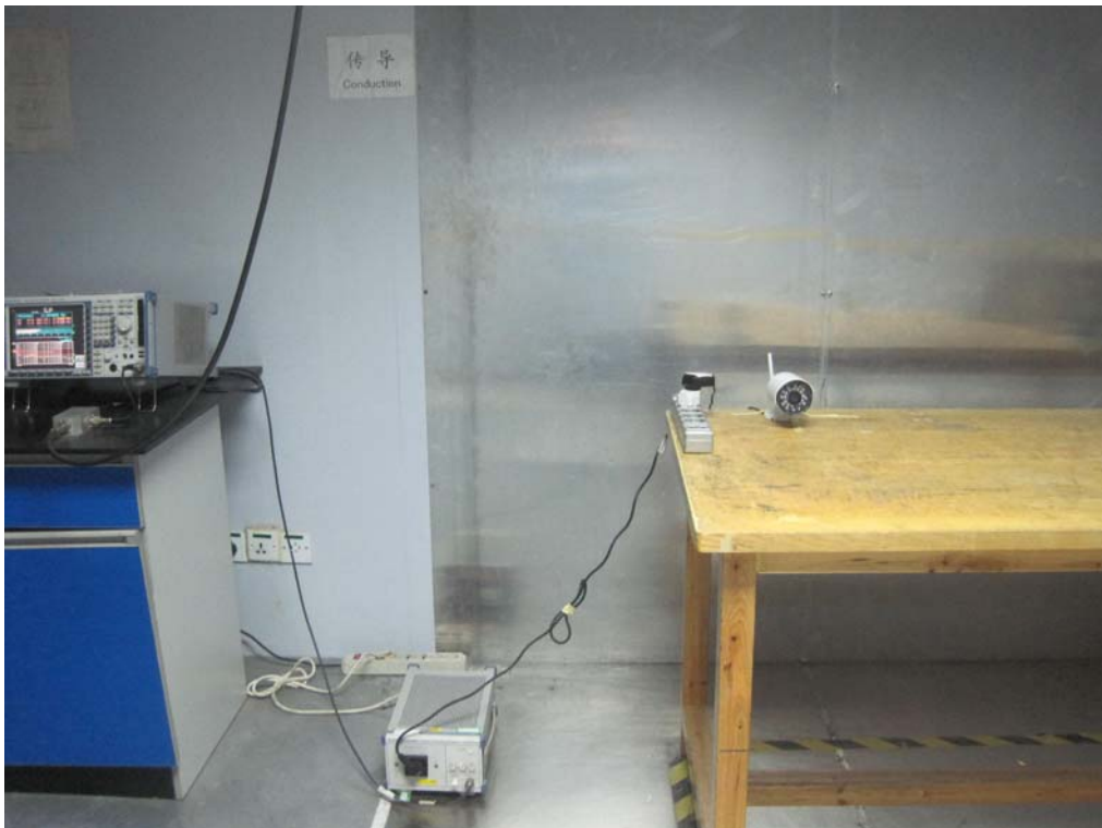
17.2 Photograph – Conducted Emission Test Setup
