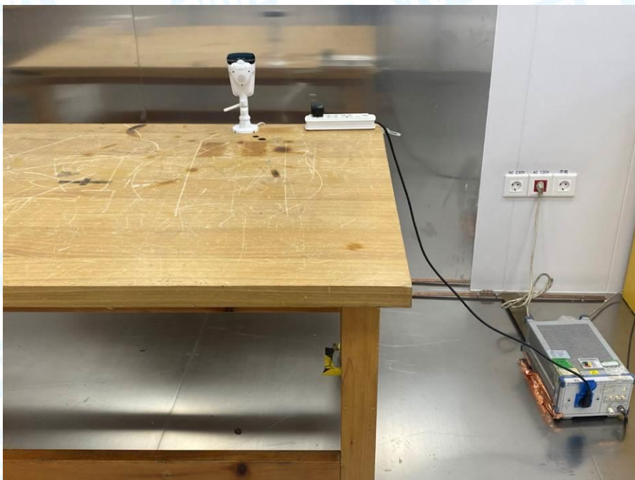
Photo of Setup for Conducted Emission
