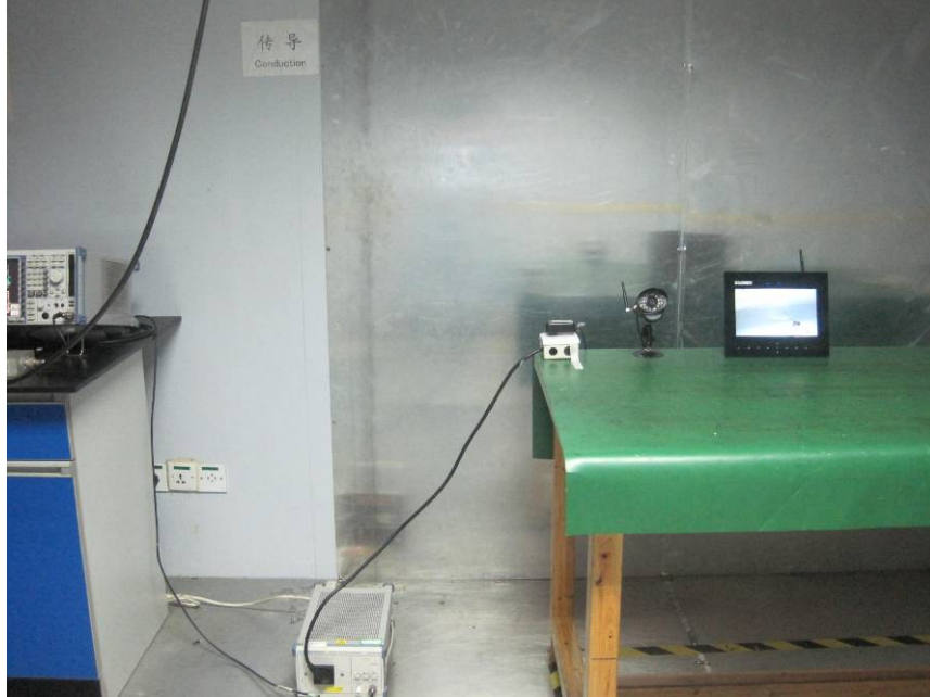
Conducted Emission Test View
