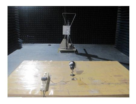
**Radiation Emission Test View For 1GHz-25GHz**
