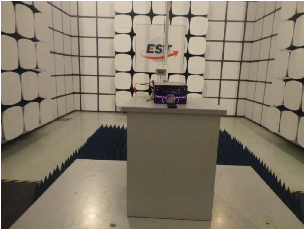
Radiated Test (1000-25000 MHz)
