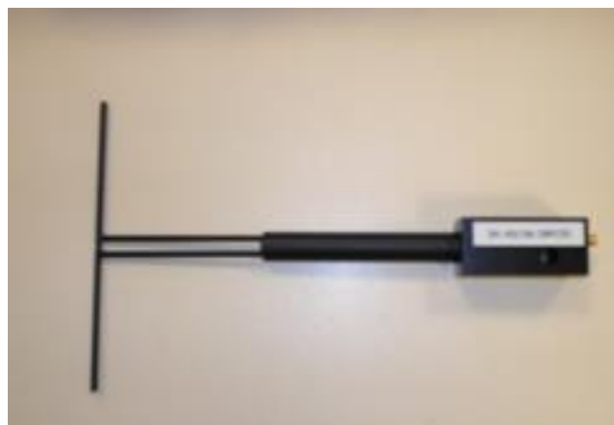
Figure 1 – MVG COMOSAR Validation Dipole
