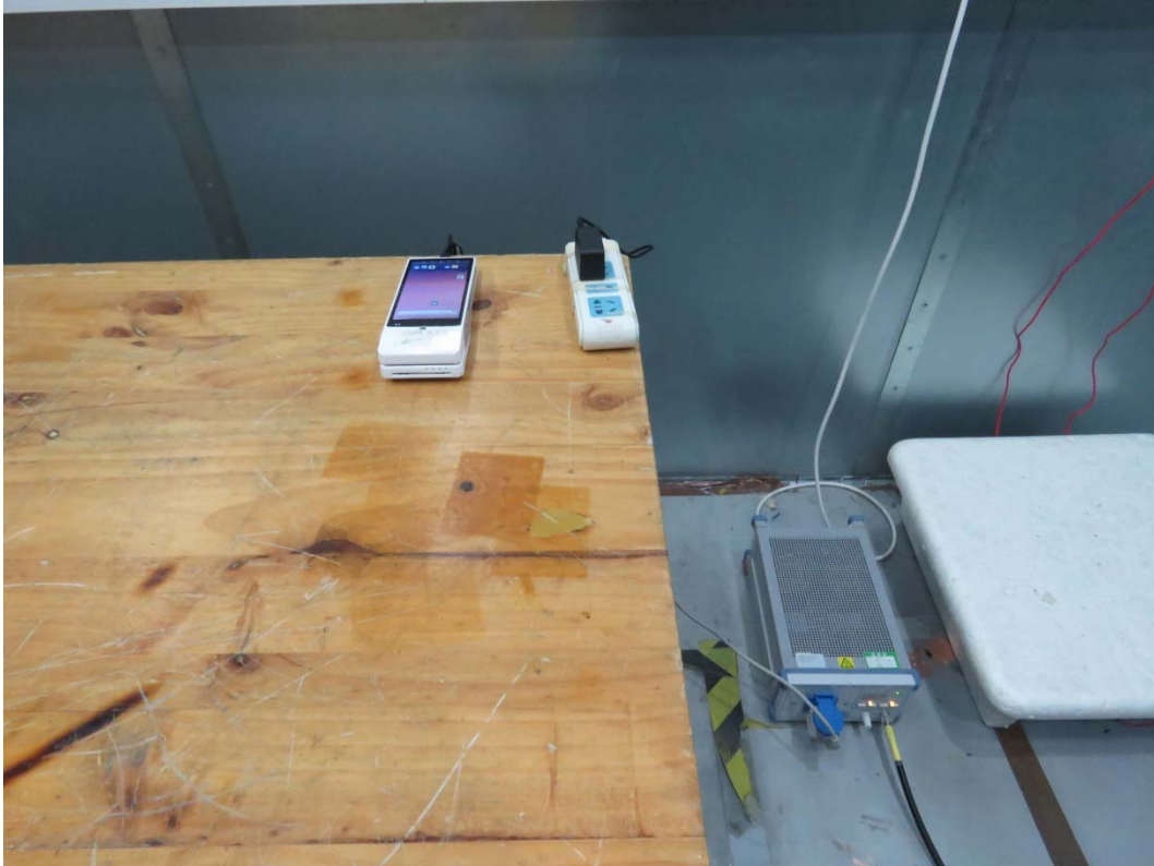
Picture 2 Conducted Emission Test Setup
