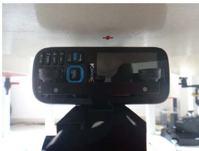
10mm Body-worn Left Side Setup Photo
