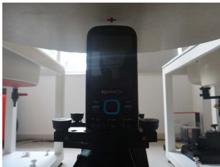
10mm Body-worn Top Side Setup Photo
