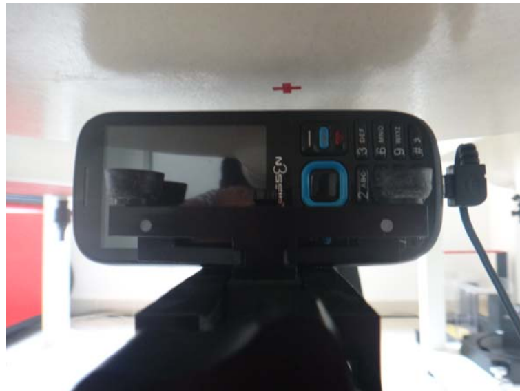
10mm Body-worn Right Side Setup Photo
