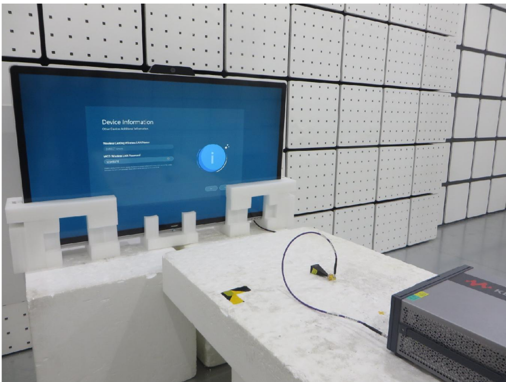
Description: Radiated Emission Test Setup for 40GHz -50GHz
