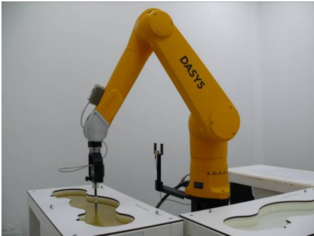
Picture 1: Specific Absorption Rate Test Layout
