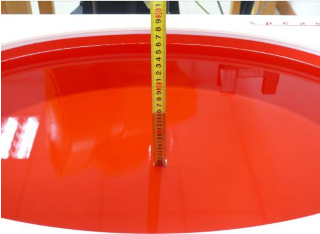
Picture 3: Liquid depth in the flat Phantom (5200 MHz, 15.4cm depth)
