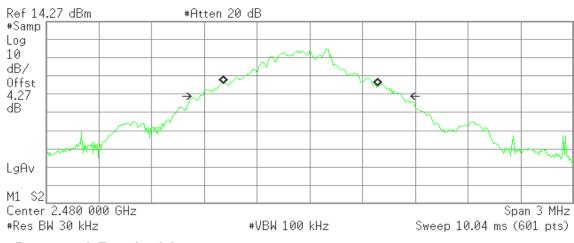
Occupied Bandwidth 870.2470 kHz Occ BW % Pwr 99.00 % x dB -26.00 dB
