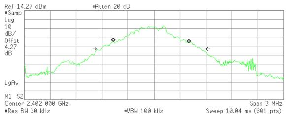
Occupied Bandwidth 868.0038 kHz Occ BW % Pwr 99.00 % x dB -26.00 dB
