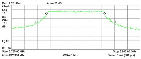
Occupied Bandwidth 18.1609 MHz Occ BW % Pwr 99.00 % x dB -26.00 dB
