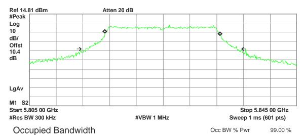
Transmit Freq Error -78.429 kHz x dB Bandwidth 22.622 MHz
