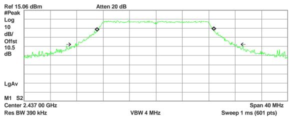
Occupied Bandwidth 17.6968 MHz Occ BW % Pwr 99.00 % x dB -26.00 dB
