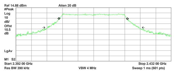
Occupied Bandwidth 17.7168 MHz Occ BW % Pwr 99.00 % x dB -26.00 dB
