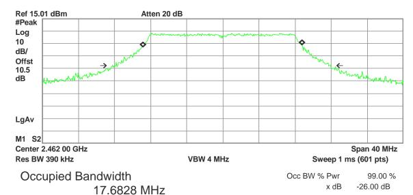
Transmit Freq Error -57.228 kHz x dB Bandwidth 24.157 MHz
