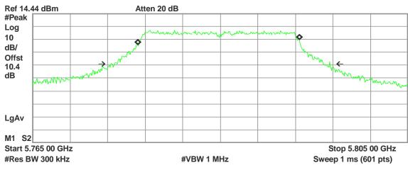
Occupied Bandwidth 17.2959 MHz Occ BW % Pwr 99.00 % x dB -26.00 dB
