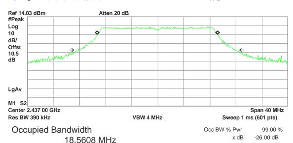
Transmit Freq Error -64.554 kHz x dB Bandwidth 24.103 MHz
