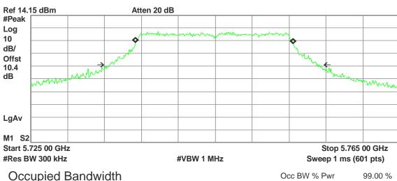
Occupied Bandwidth 17.1668 MHz Occ BW % Pwr 99.00 % x dB -26.00 dB
