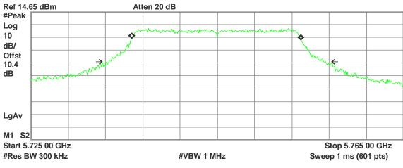
Occupied Bandwidth 18.2117 MHz Occ BW % Pwr 99.00 % x dB -26.00 dB
