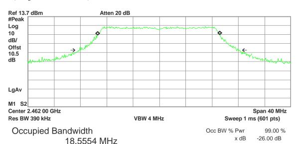
Transmit Freq Error -91.035 kHz x dB Bandwidth 24.092 MHz
