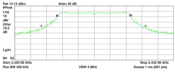
Occupied Bandwidth 18.5479 MHz Occ BW % Pwr 99.00 % x dB -26.00 dB
