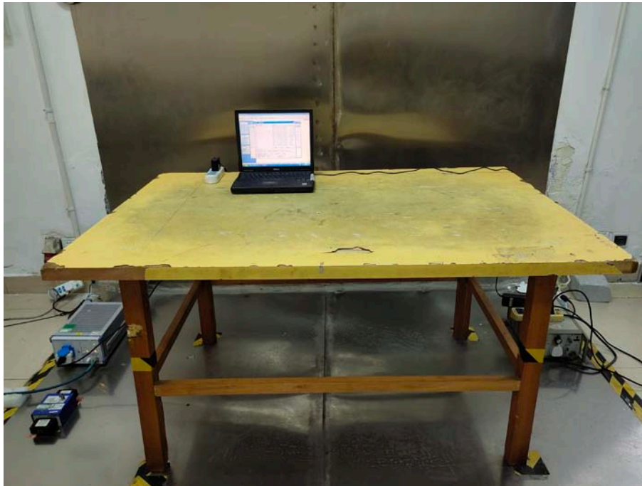
Conducted Emission Test Setup Front View
