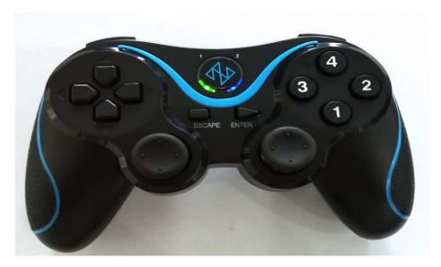
1. Press the power key until green light turns on and blue light flash. This is pairing status..
