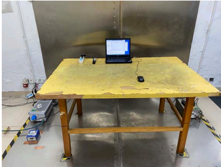
Conducted Emissions Test Setup Front View
