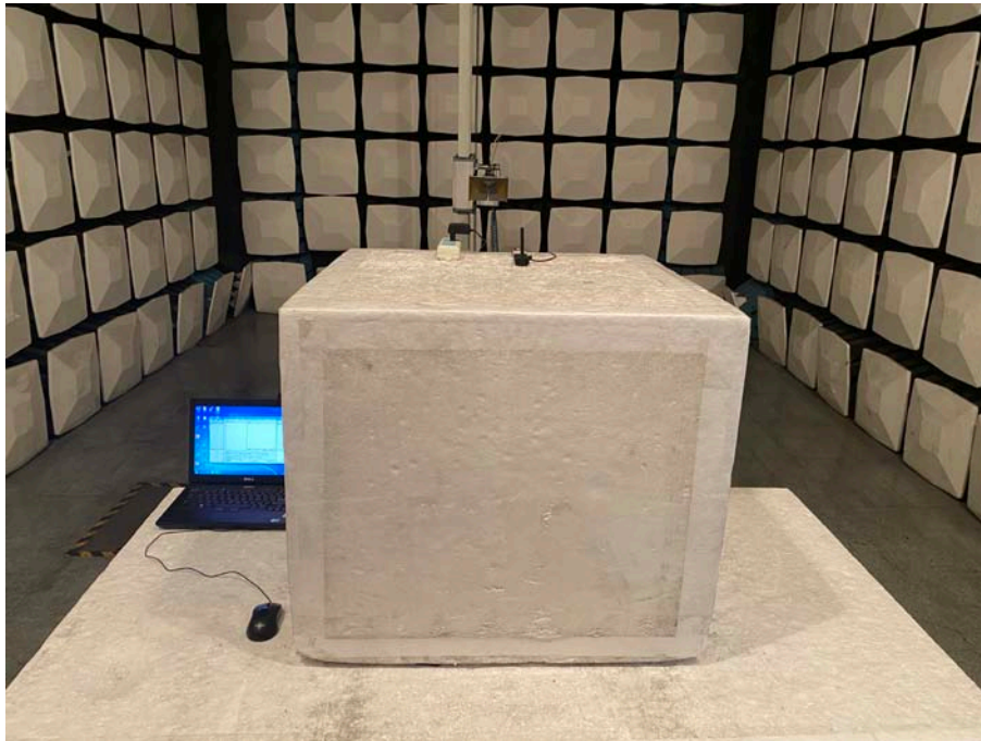
Radiated Emission Front View (Above 1GHz)
