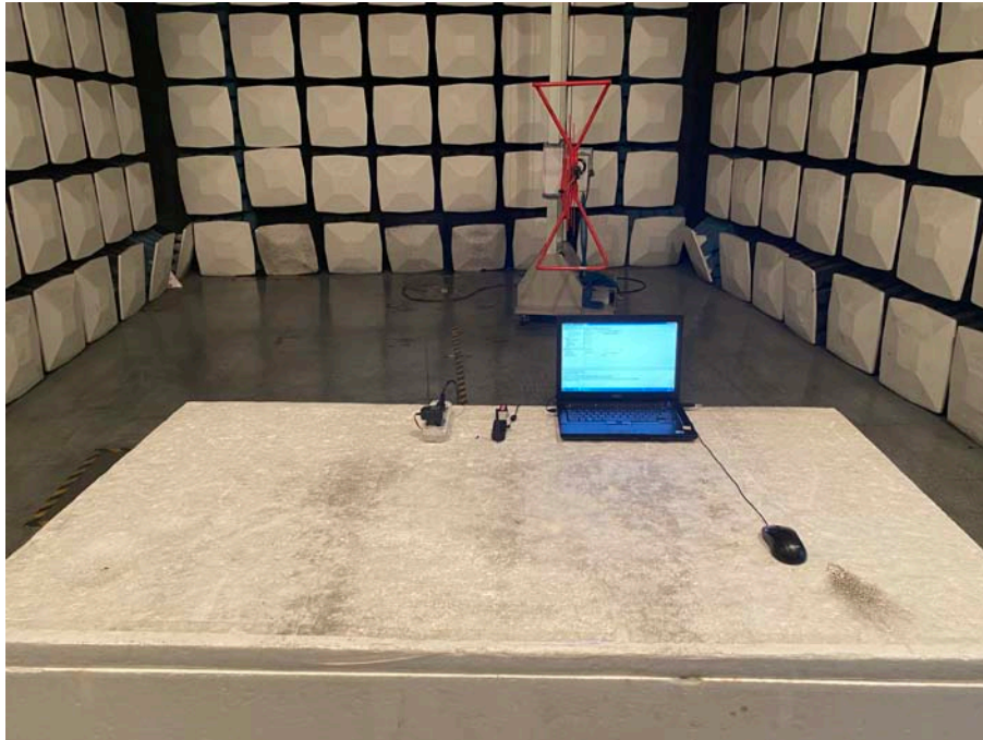
Radiated Emission Front View (Below 1GHz)
