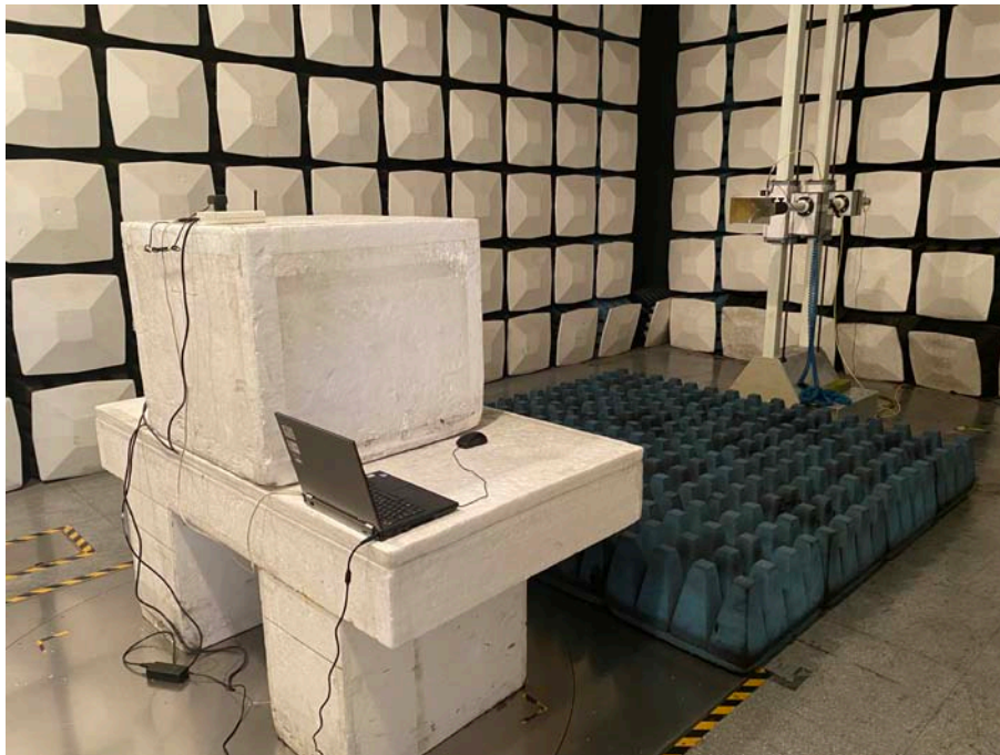
Radiated Emission Rear View (Above 1GHz)
