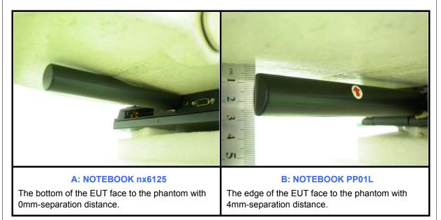
**NOTE:** The bottom of the notebook contacts to the bottom of the flat phantom with 0mm-separation distance.
