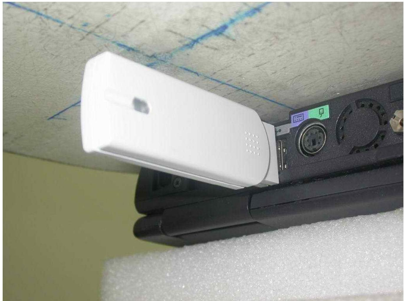
**The Bottom of the EUT to the flat phantom distance 10 mm**
