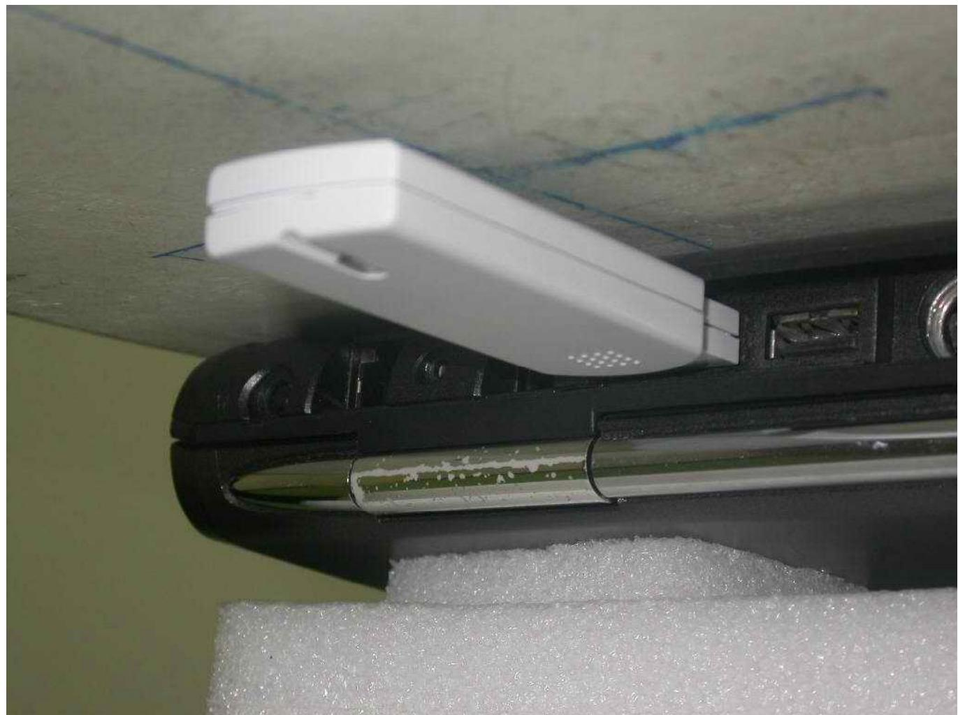
**The Bottom of the EUT to the flat phantom distance 9 mm**
