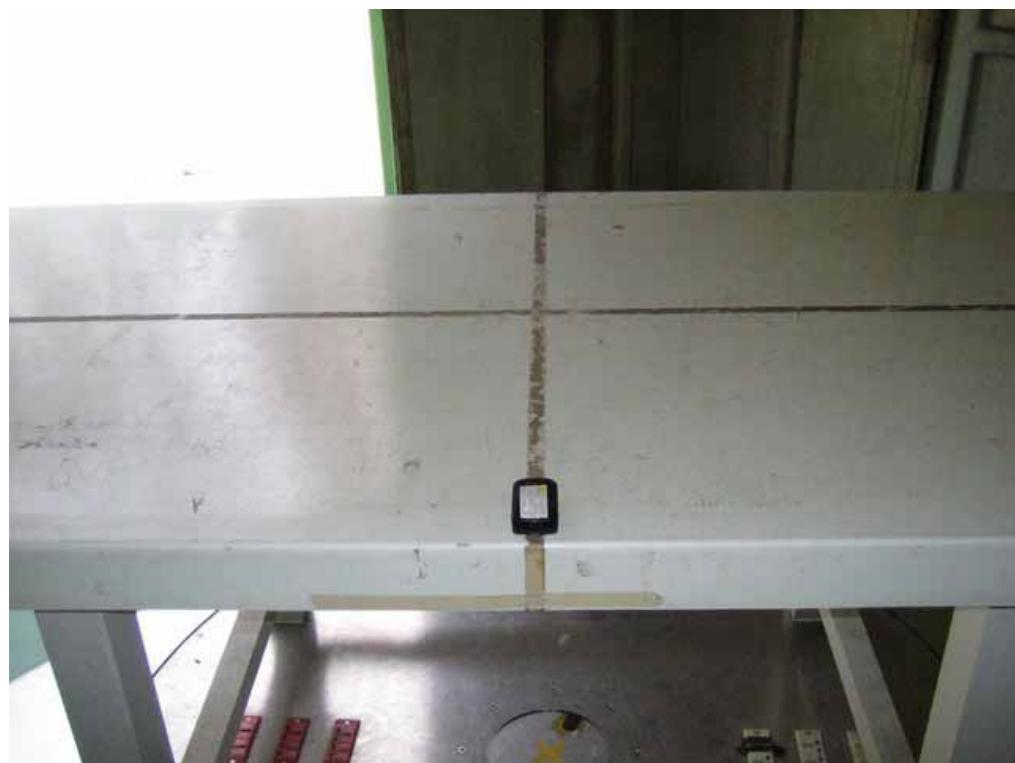
**RADIATED RF MEASUREMENT SETUP**
