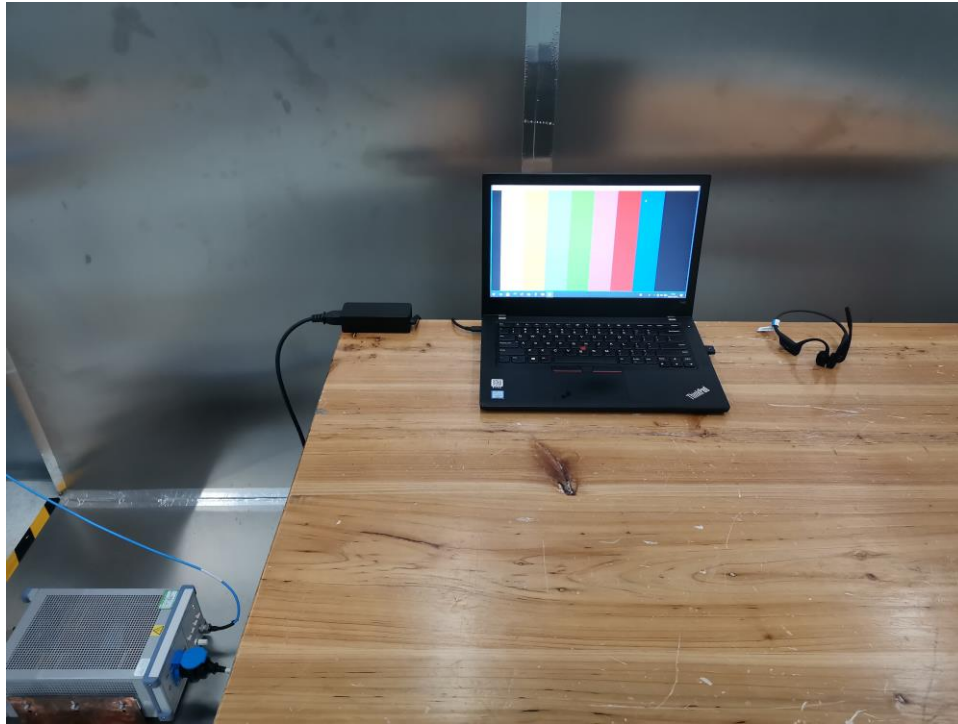
Photograph 3: Set-up photo for Conducted Emission
