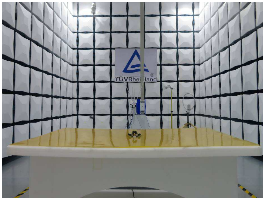
Photograph 1: Set-up for Radiated Spurious Emission, Below 1GHz
