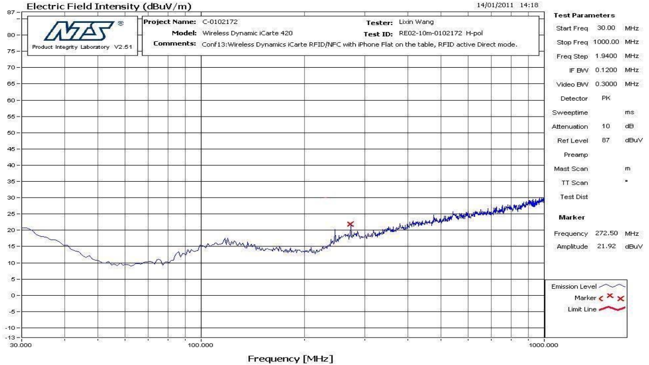
Figure 12 30 MHz to 1000 MHz Vertical Direct mode at 10m distance
