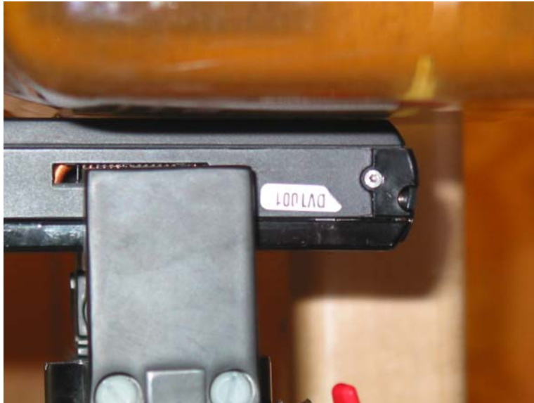
WLAN Main Antenna Position
