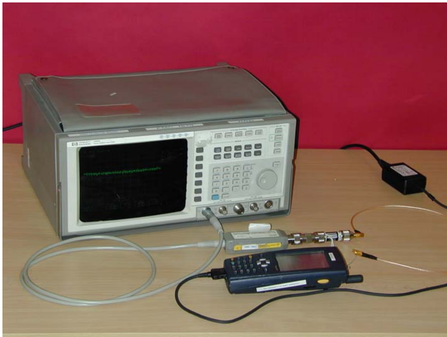
Figure 4. Photograph of test set-up used for obtaining statistics on peak and average power
