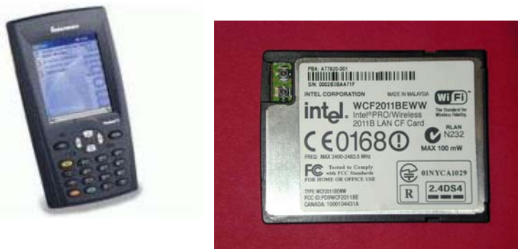
Figure 1. The test device employed as a DSSS source showing Intermec Pocket PC and Intel LAN card
