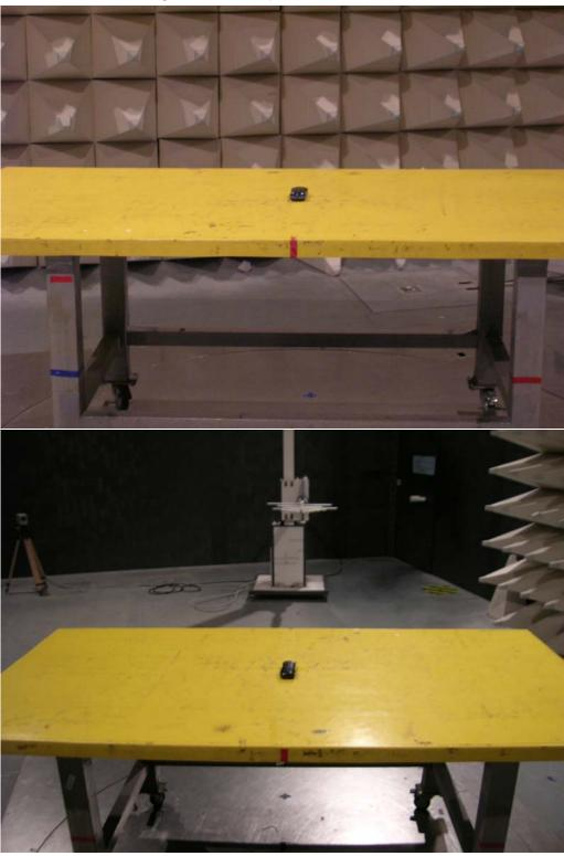
Radiated Emissions (1GHz~10<sup>th</sup> harmonic of highest frequency)
