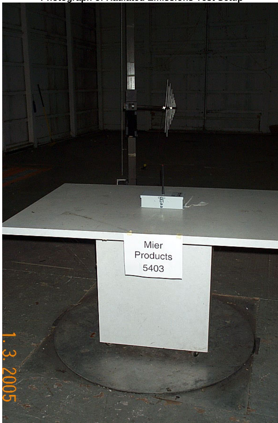
Photograph of Radiated Emissions Test Setup
