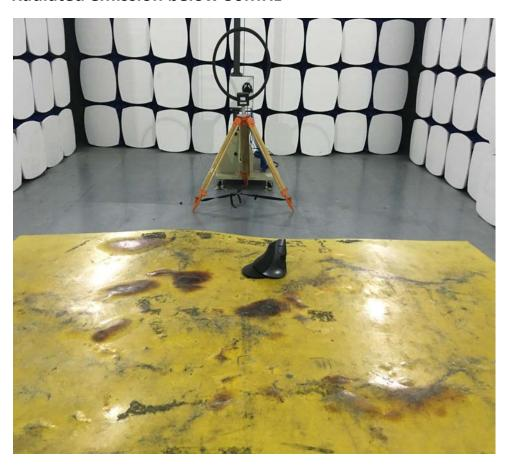
Radiated emission 30MHz to 1GHz
