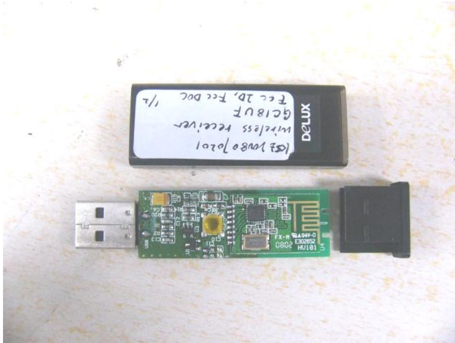
Main board component side
