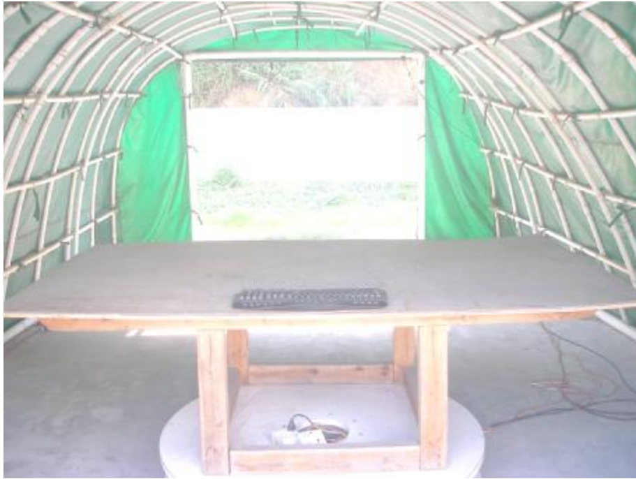
Radiated emission test view
