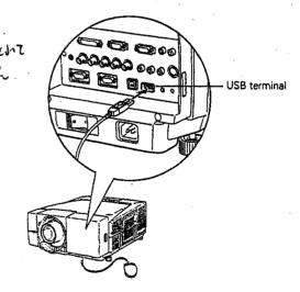
Connect the USB terminal on the projector and a USB mouse when operating the projector with the USB mouse. A mouse cursor will appear on the screen with the mouse connected.
