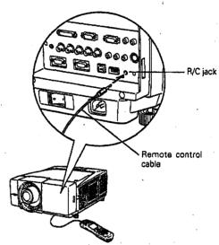
Connect the R/C JACK on the projector and the remote control with the remote control cable when operating the remote control with wired.
