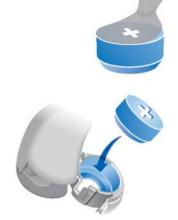
Carefully close the battery compartment. If you feel resistance, the battery is not inserted correctly.
