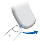
Lightly tap the instrument or use the magnet stick to remove the battery. The magnet stick is available as an accessory.
