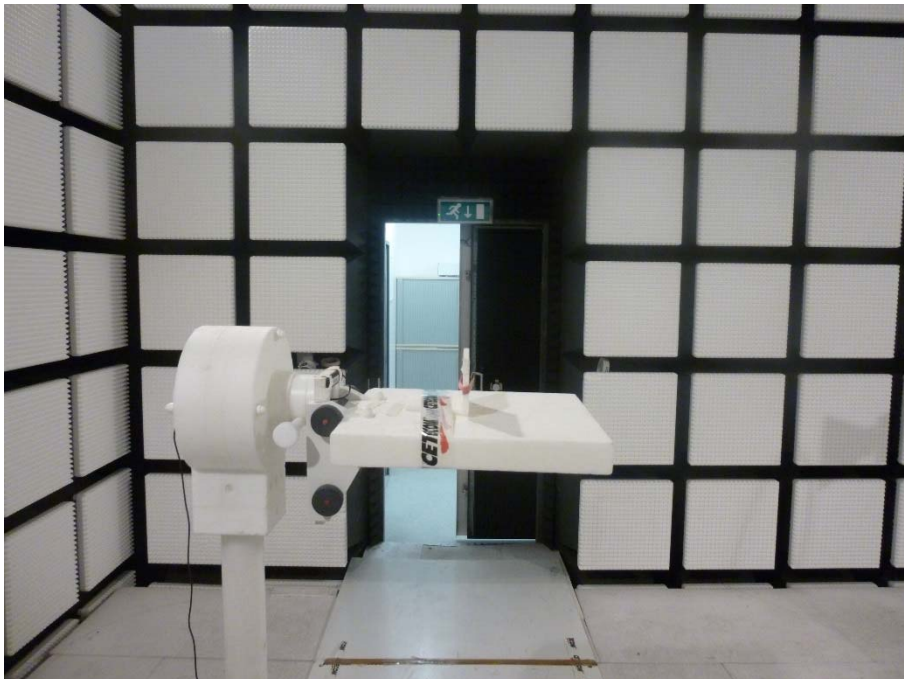
Photo 4: EUT at the anechoic chamber
