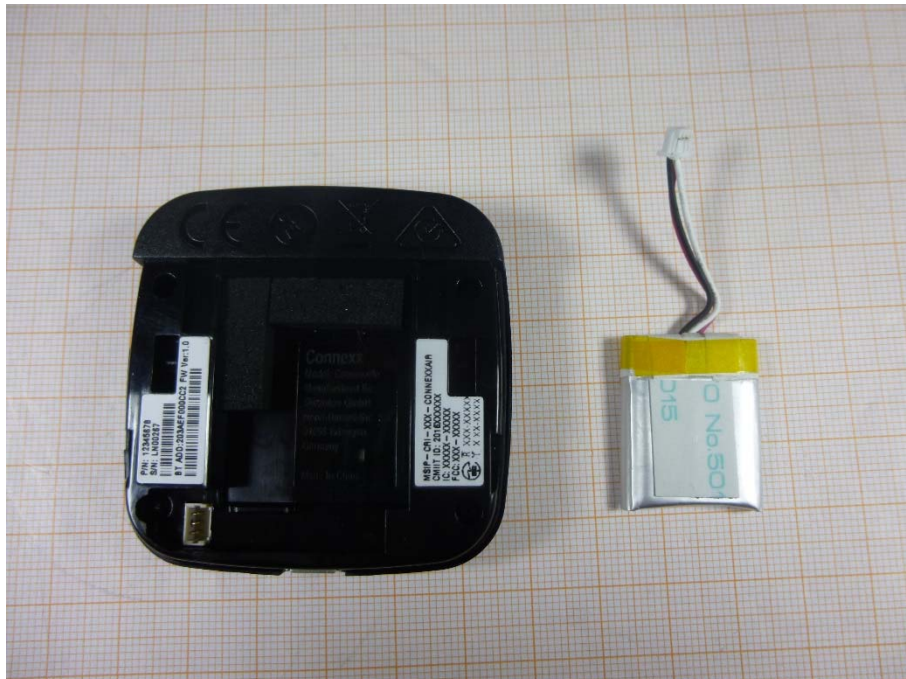
Photo 2: Battery pack removed
