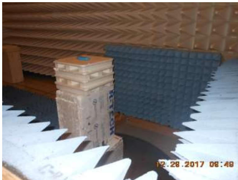
Above 1GHz, Cone Placement
