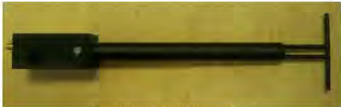
Figure 1 – MVG COMOSAR Validation Dipole
