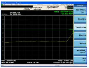
Conducted Band Edge plot on channel 4233
