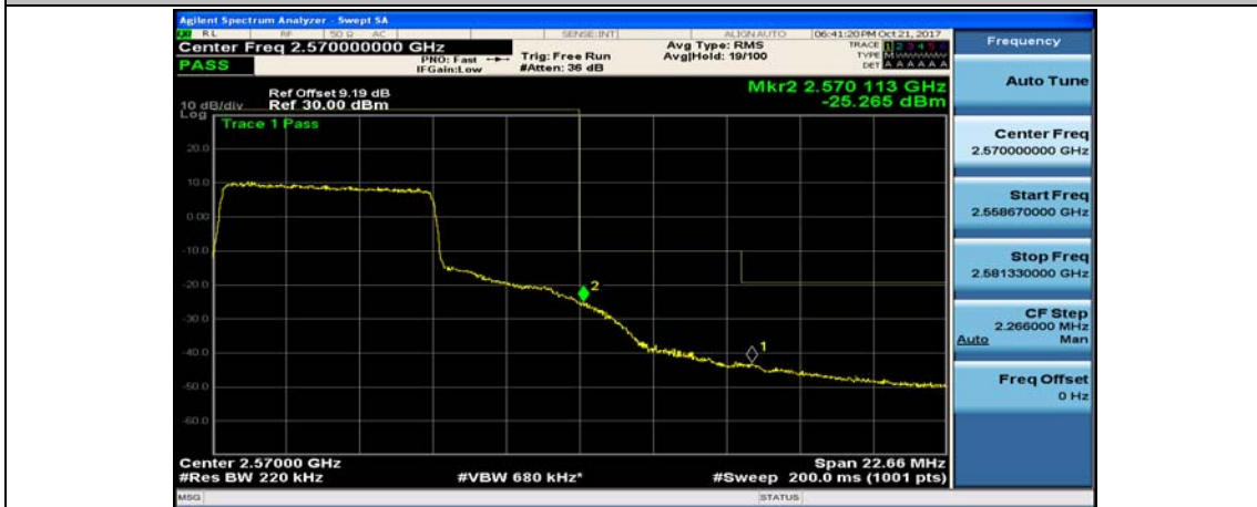
(Channel Bandwidth:15 MHz)_HCH_16QAM_37RB#38
