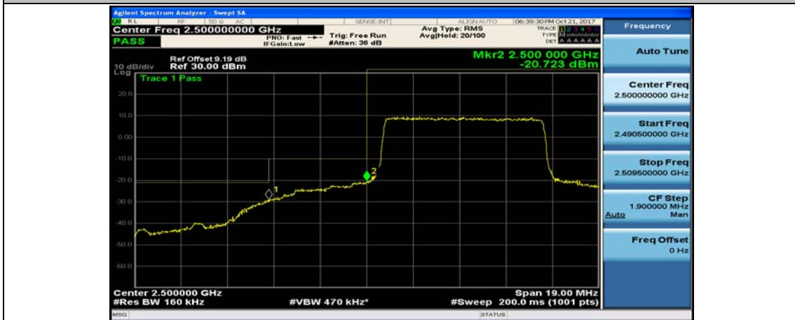
(Channel Bandwidth:15 MHz)_LCH_16QAM_37RB#18
