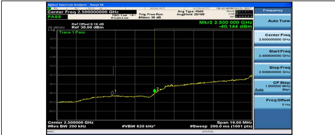
(Channel Bandwidth:20 MHz)_LCH_QPSK_100RB#0
