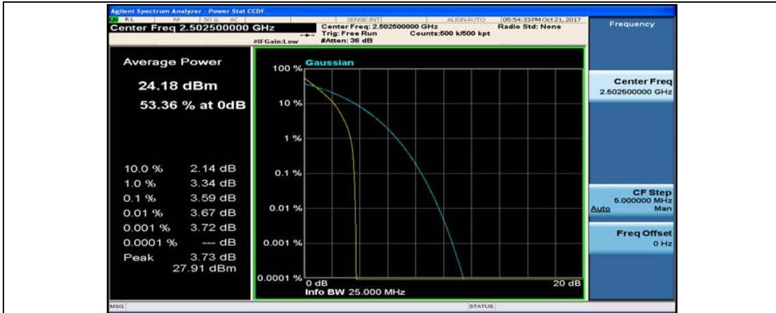
(Channel Bandwidth: 5 MHz)_LCH_QPSK_12RB#6
