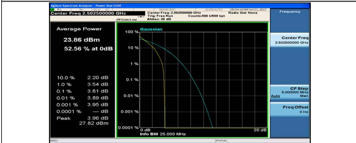
(Channel Bandwidth: 5 MHz)_LCH_QPSK_25RB#0
