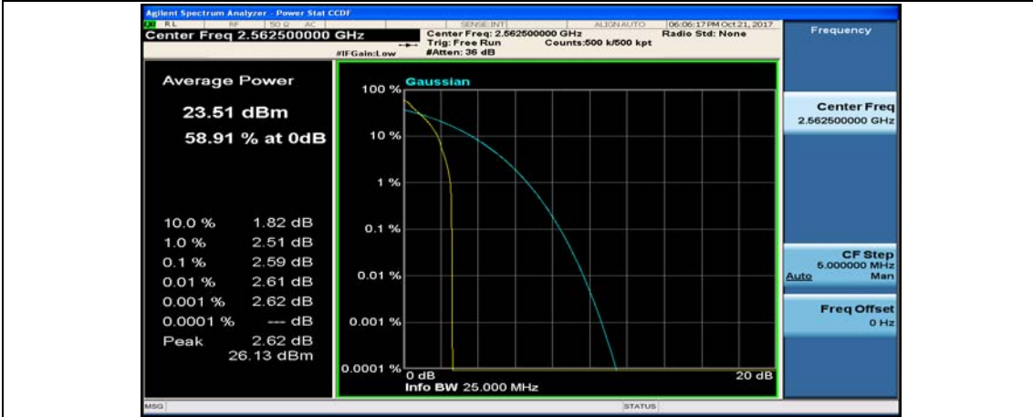
(Channel Bandwidth:15 MHz)_HCH_QPSK_1RB#74
