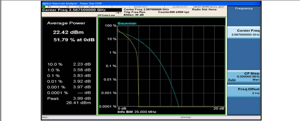
(Channel Bandwidth: 5 MHz)_HCH_QPSK_25RB#0
