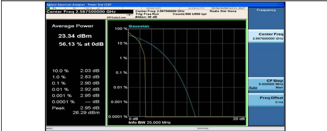
(Channel Bandwidth: 5 MHz)_HCH_QPSK_1RB#12
