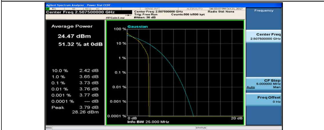
(Channel Bandwidth:15 MHz)_LCH_QPSK_37RB#0
