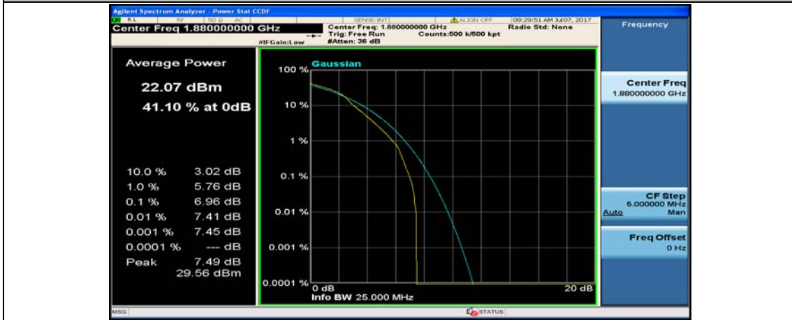
Channel Bandwidth: 10 MHz_MCH_16QAM_1RB#49
