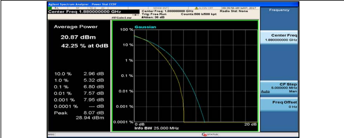
(Channel Bandwidth:20 MHz)_MCH_16QAM_100RB#0
