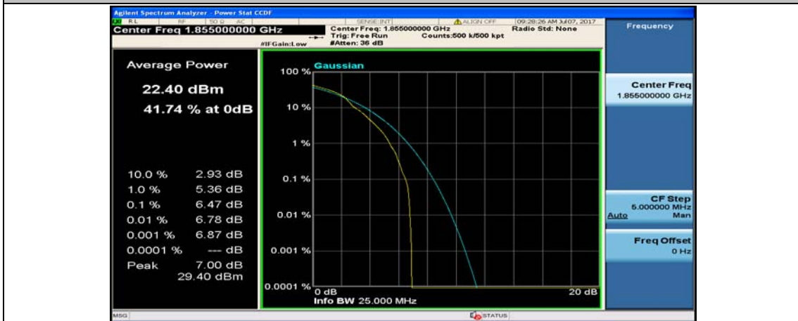
Channel Bandwidth: 10 MHz_LCH_16QAM_25RB#0
