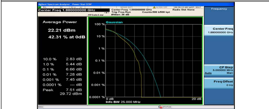
(Channel Bandwidth:20 MHz)_MCH_16QAM_1RB#99
