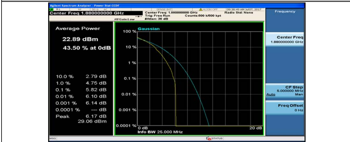
(Channel Bandwidth:20 MHz)_MCH_QPSK_1RB#49
