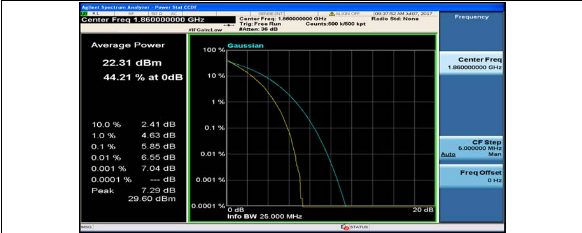
(Channel Bandwidth:20 MHz)_LCH_QPSK_50RB#25
