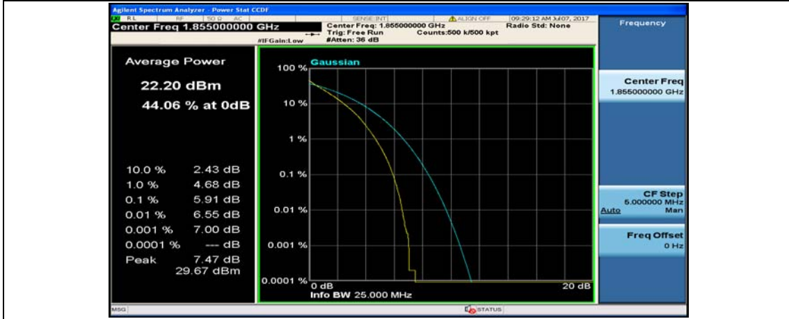
Channel Bandwidth: 10 MHz_MCH_QPSK_1RB#0
