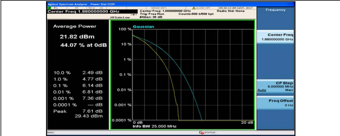
Channel Bandwidth: 10 MHz_MCH_QPSK_50RB#0
