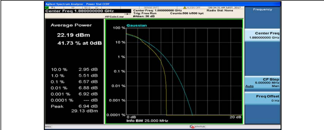
(Channel Bandwidth:15 MHz)_MCH_16QAM_37RB#0
