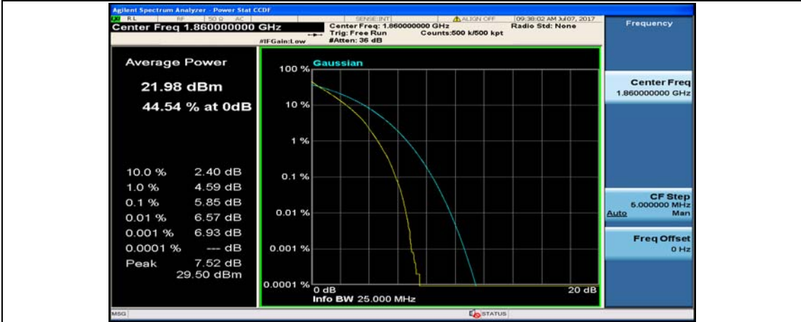
(Channel Bandwidth:20 MHz)_LCH_QPSK_100RB#0
