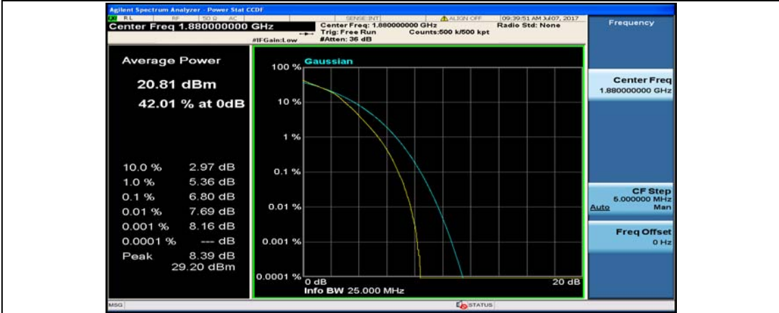
(Channel Bandwidth:20 MHz)_MCH_16QAM_50RB#50
