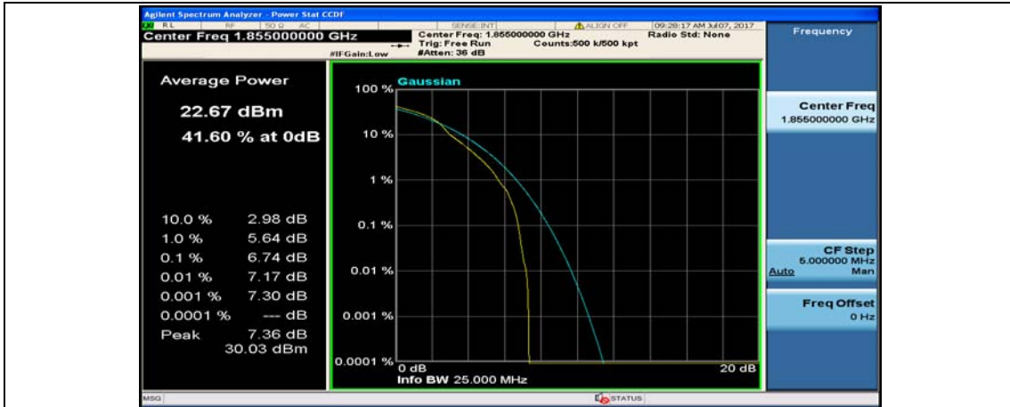
Channel Bandwidth: 10 MHz_LCH_16QAM_1RB#24
