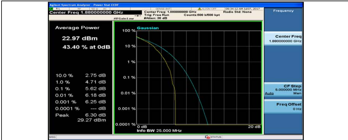
(Channel Bandwidth:15 MHz)_MCH_QPSK_37RB#0
