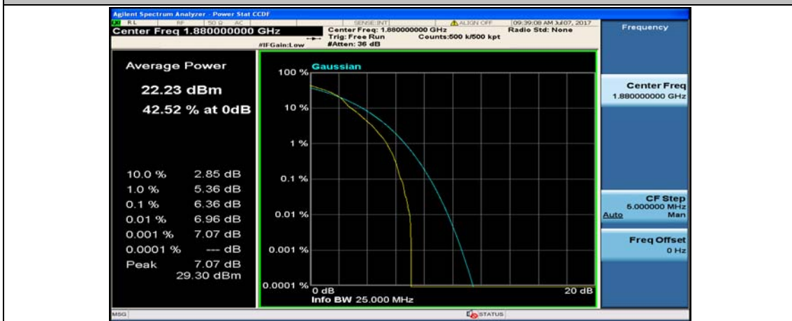
(Channel Bandwidth:20 MHz)_MCH_16QAM_1RB#49
