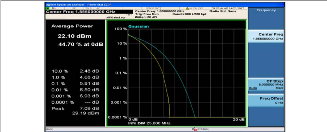
Channel Bandwidth: 10 MHz_LCH_QPSK_50RB#0
