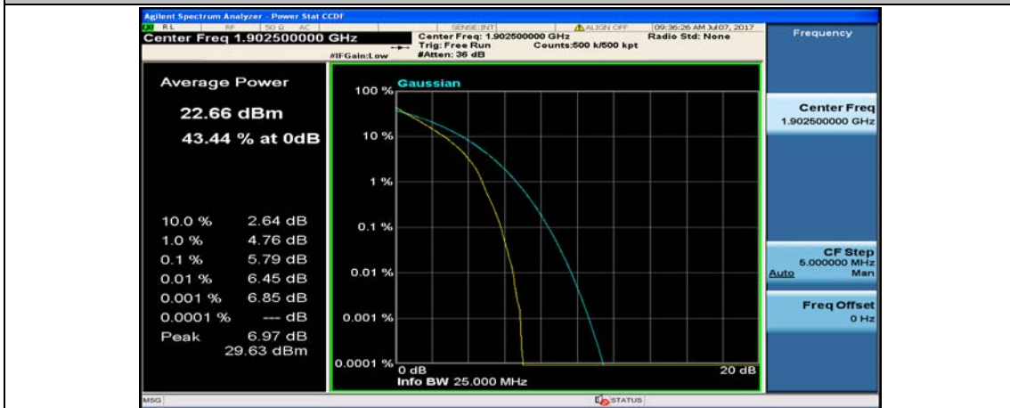
(Channel Bandwidth:15 MHz)_HCH_QPSK_75RB#0
