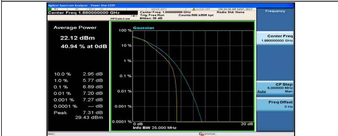
(Channel Bandwidth:15 MHz)_MCH_16QAM_1RB#74
