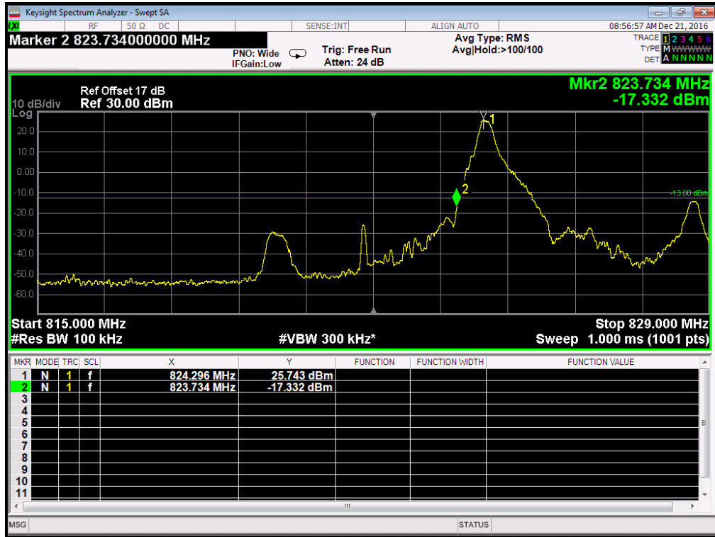
Lower Band Edge Plot for 16QAM -RB Size 1, RB Offset 0
