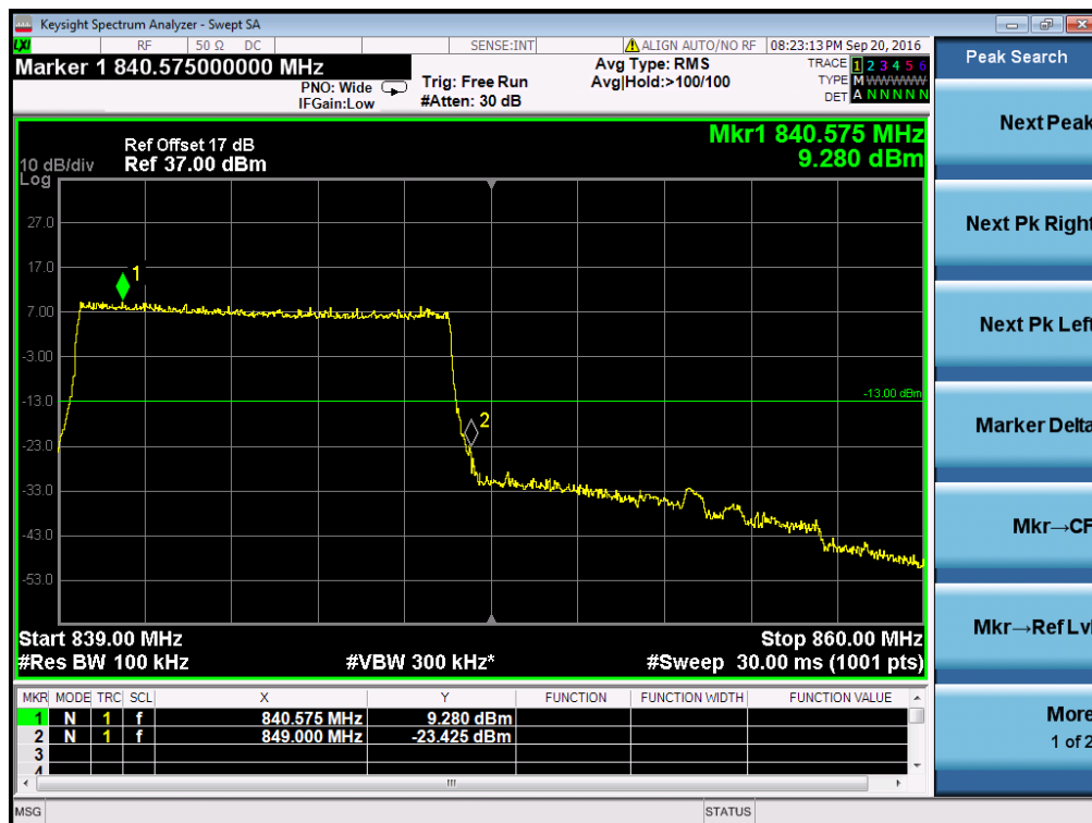
Higher Band Edge Plot for QPSK-RB Size 50, RB Offset 0
